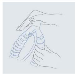
Figure 4-5. Circuit Wye Piece Obstruction
