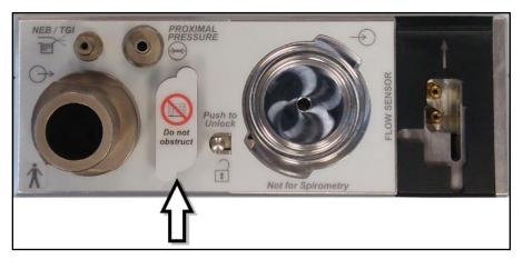
Figure 3-7. Side panel detail – safety valve intake.
