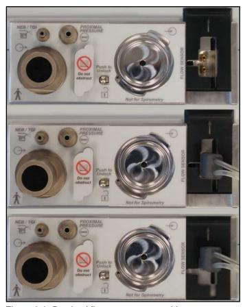
Figure 3-8. Proximal flow sensors assembly
