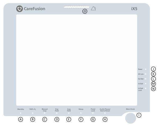
Figure 5-1. User interface, showing buttons and LEDs
