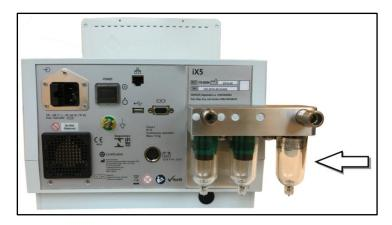
Figure 3-4. Gas intake filters
