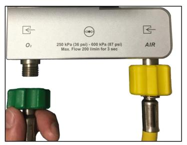
Figure 3-3. Connection of the air and oxygen hoses
